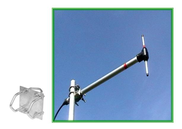
The CF5U is designed to withstand the harshest environment. Made of foam filled rigid aluminium with the radiating elements sealed within an epoxy resin filled body. The N type connector is covered with a waterproof shroud to seal any cables the antenna connects to.
